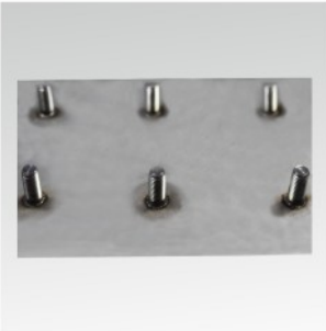
螺柱焊不锈钢板 Studs welded on stainless steel plate
